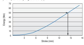
Force stroke characteristic curve (dynamic) (With impact velocity range over 0.5 m/s)
