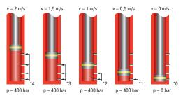
\* The load velocity reduces continuously as you travel through the stroke due to the reduction in the number of metering orifices (\*) in action. The internal pressure remains essentially constant and thus the Force vs. stroke curve remains linear.
