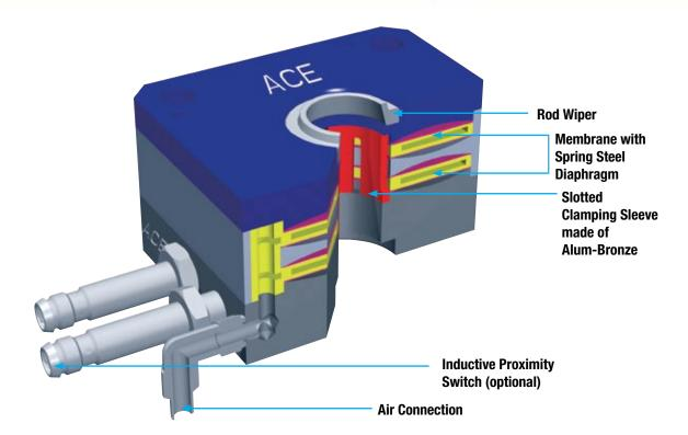
The innovative LOCKED SERIES Type P offers pneumatic rod clamping in both directions of movement for rod diameters of 16 mm up to 50 mm. The values of hydraulic clamping are met and exceeded at holding forces of up to 27,000 N.
