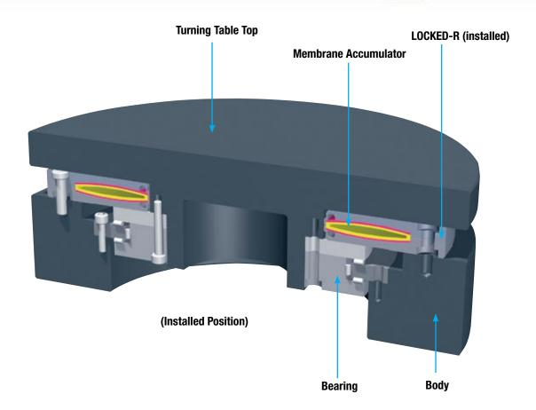
ACE's innovative pneumatic clamping elements of the LOCKED SERIES Type R offer the highest forces and holding for clamping of rotational movements directly on the shaft. They are available in standard sizes for shaft diameters of 50 to 340 mm. Due to the spring-brake actuator principle, energy failure is immediately followed by safety clamping.
