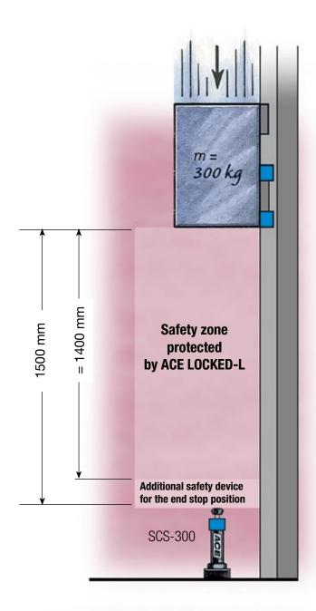
In the example shown above the final 1500 mm linear travel of the carriage is protected by the use of two ACE LOCKED Type L clamping elements. If automatic clamping of the axis, eg. by a power failure, is not available then the free falling mass of 300 kg is braked safely in a stopping distance of approx. 100 mm. This stopping distance is additionally protected at the end position by a small safety shock absorber from ACE Controls.
