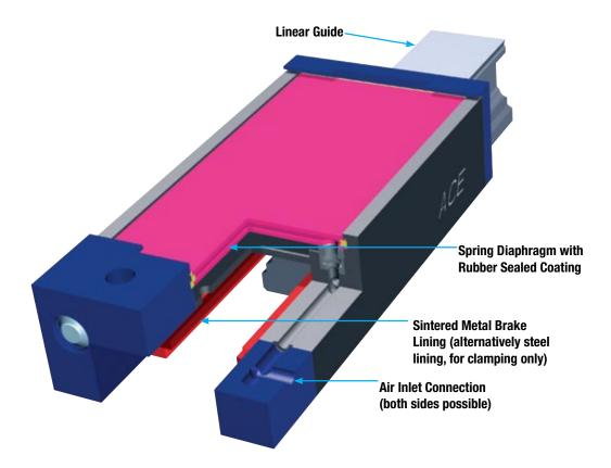
The innovative pneumatic clamping elements of the new ACE LOCKED SERIES Type-L offer a safe clamp/or brake system fitted directly on the guided rail. They are suitable for the majority of all rail sizes and manufacturers, such as INA, STAR/Rexroth, THK, Schneeberger and many others.
